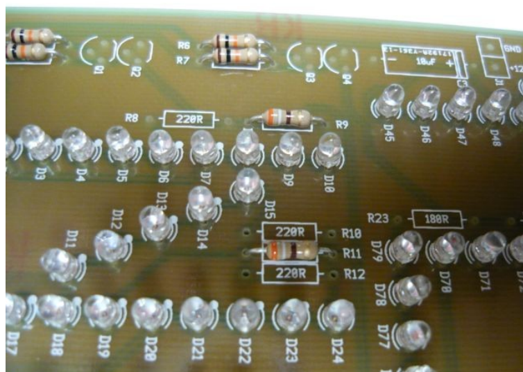
Illustration 12: Resistor 390 \Omega (R9, R11)
