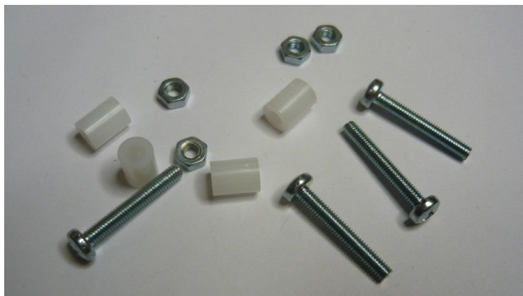
Illustration 30: 20mm screws and nuts and spacers
