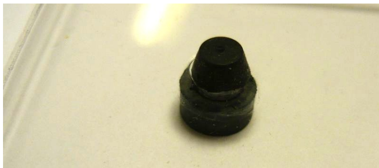
Illustration 34: Rubber foot through base-plate
