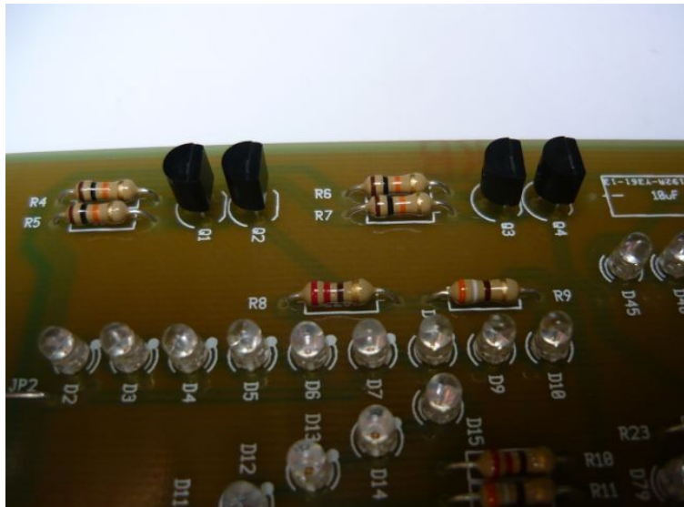
Illustration 20: Transistors BC337 (Q1..Q4)
