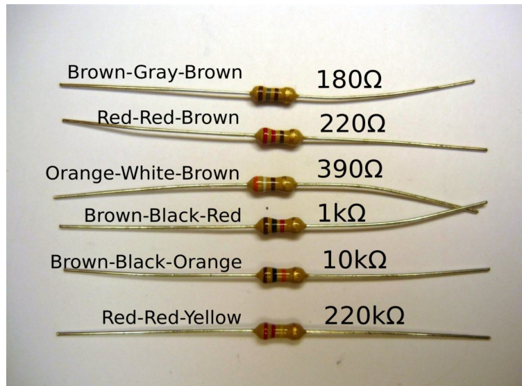
Illustration 7: Resistor values and colors
