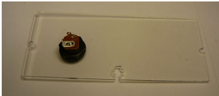
Illustration 27: Connector screwed into back plate
